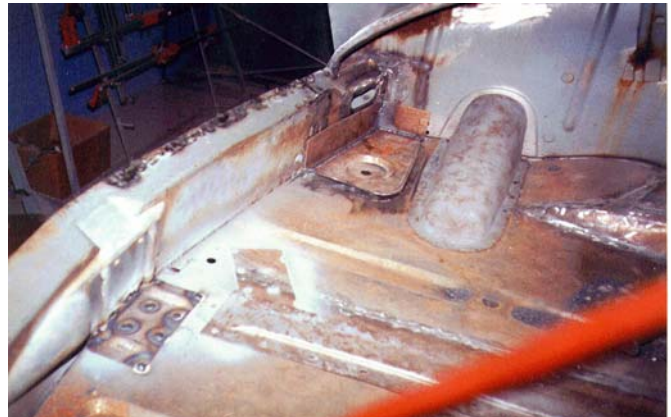
Welding the Trunk
