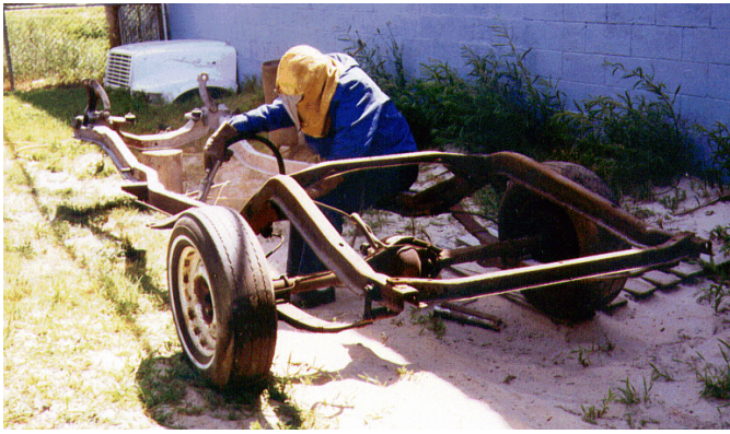
Sand Blasting the Frame
